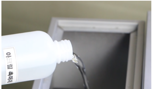
(4) Add catalyst at A agent, and mix each other using a stick.
