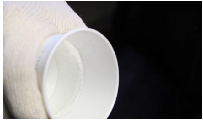
(7) Checking hardening time(c): if hardening time is long, increase the catalyst in order to shorten.
